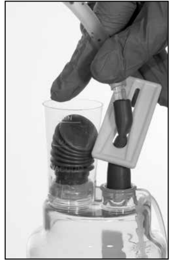
Opening sliding clamp on green connection tubing
