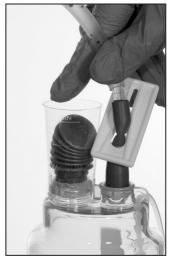
Opening sliding clamp on green connection tubing
